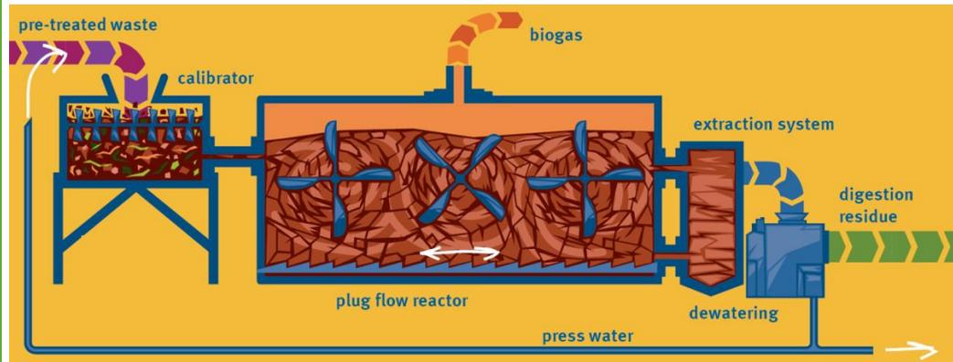
Digestion processes are completed after about 18–21 days and the remains dewatered in a press. The solid matter can then be further cured by composting and deposited at landfills whereas the waste water has to undergo further treatment. Due to the high COD, expensive methods for the treatment of the waste water have to be employed, however.
